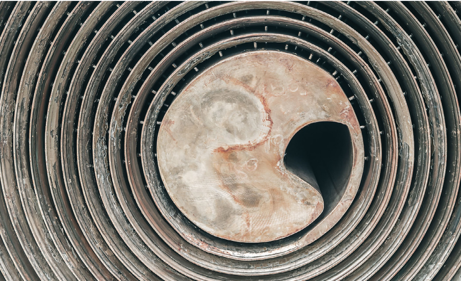
Spiral heat exchangers can be difficult to clean and maintain
