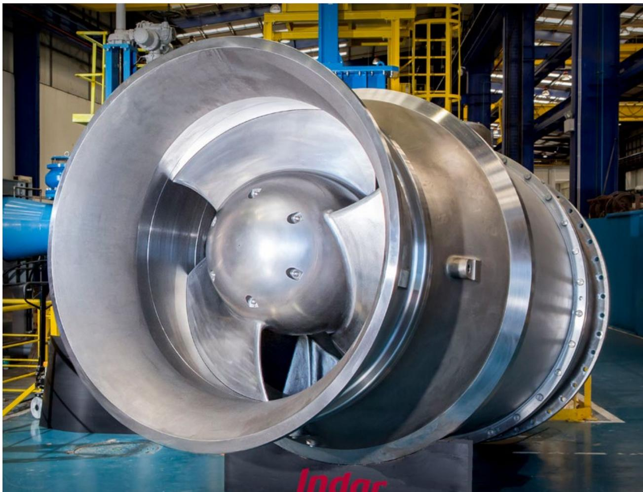
H-1800-1697 +S-450-X/8 Motorpump set, Fishfriendly design. Impeller view
